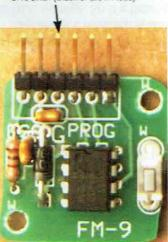
a profile model; others with a fuselage model will use the FM-9 with the start button replaced with a remote start button on 6" leads. Other timer boards include the FM-9R which has a BEC circuit for ESCs that don't provide the 5 volts needed by the timer. There are also some timers that add control of retractable landing gear, FM-9V timers uses a pot to vary the RPM around the programmed value, etc.
